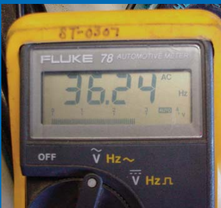
Figure 2: The ignition system's 3X signal was verified by attaching a DMM, set to measure frequency (Hz).
