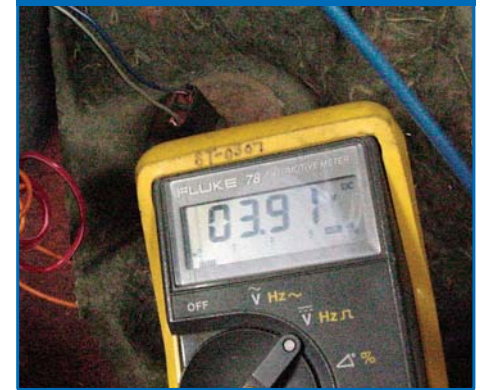
Figure 5: 3.91 V won't energize the fuel pump relay. Time to identify the source of the voltage drop.
