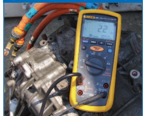
Figure 5: Second transaxle with good MG windings
