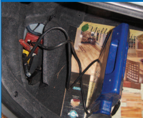
Figure 2: Installing battery pack on AGM battery
