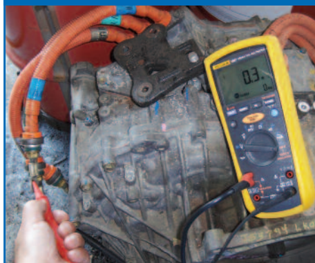
Figure 4: Hybrid transaxle with shorted MG windings
