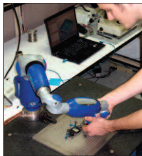
The use of integrated mobile measurement equipment allows greatly improved measurement accuracy during the part manufacturing process.
