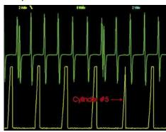
On certain types of GM control modules, including this one, the point the transistor is turned on is determined by the module, based upon the input data it receives. The point the transistor is turned off is determined by the ECM through the EST signal. It's what is between those two points that is really interesting. The dwell time or actual coil primary winding charge time is determined to a great extent by the coil inductance. Inductance
