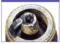
This disadvantage could be avoided if the knock limit were determined continuously during operation. The ignition advance then could be continuously adjusted, in a closed loop operation, just below the point where knock begins. The only problem is, how do we let the control unit know when the engine has begun to knock?
