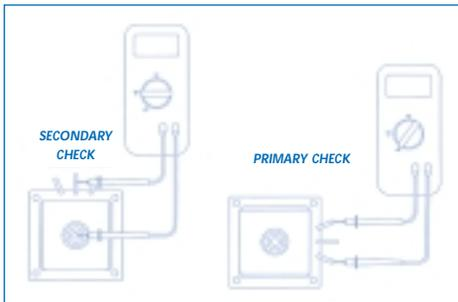
**NOTE:** Before you measure the primary resistance in any coil, you should always "baseline" the ohmmeter by touching the two test leads together to see how much resistance is in the leads. Then remember to subtract this amount from the actual coil reading to accurately measure the coil's primary resistance. Forget this step and a bad coil may test good or vice versa.
