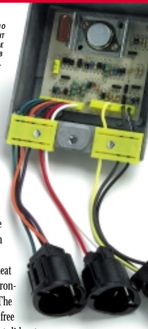
current limiters. New cooler running, longer lasting transistors were also added to improve reliability. The electronics were also embedded in an improved potting material for better heat dissipation and environmental protection. The result was a trouble-free replacement unit that did not suffer repeat failures like the OE unit.
