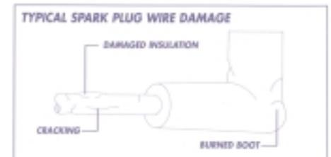
Loose-fitting spark plug boots or damaged insulation on the plug wires may also provide paths where the spark can escape to ground. Good plug wires should generally have less than 8,000 ohms per foot resistance. If resistance exceeds specifications, or the plug wires are found to be damaged, replace the wires.
