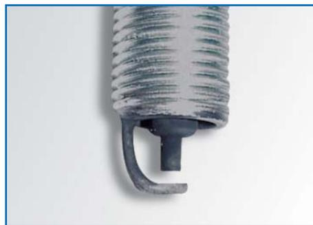
Damaged Spark Plug
