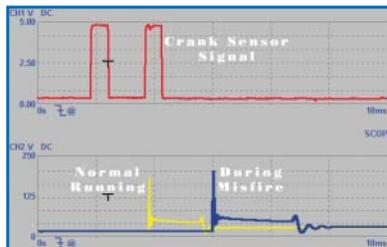
The crank sensor on this engine is mounted on the bellhousing and produces its signal from the flywheel rotation. This signal should remain constant unless the crank sensor is defective or something happens to the flywheel to change the timing of the signal. After looking at the two patterns, I could see the ignition timing had changed under the same engine rpm and load. The computer, a defective crankshaft position sensor or something mechanical could cause this.
