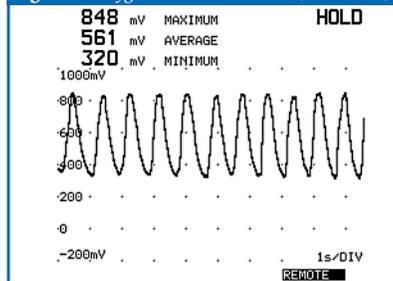
signal amplitude. If the oxygen sensor response has deteriorated, it will show reduced amplitude. If the calibrated frequency could not be obtained while running the test due to excessive purge vapors, the test will be run again.
