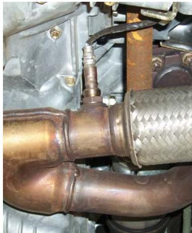
As described in the last *Counter Point*, some OBD II systems monitor the operation of the oxygen sensor heaters *indirectly* with a deductive test. The heater is used along with the oxygen sensor to permit the powertrain control module (PCM) to convert to closed loop operation as soon as possible after engine start-up. If the oxygen sensor begins producing a useable signal within the prescribed period after engine start-up, the oxygen sensor heater monitor is satisfied.
