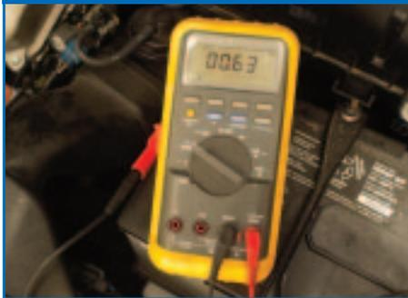
To measure a four-wire A/F sensor's response using *amperage*, install an ammeter *in series* with the PCM's 3.3 volt signal wire. The ammeter's negative (black) lead should be connected to the sensor lead and the positive (red) lead should be connected to the PCM wiring. The 3.0 volt signal wiring as well as the heater wires must remain connected (jumped between connectors) during this test.
