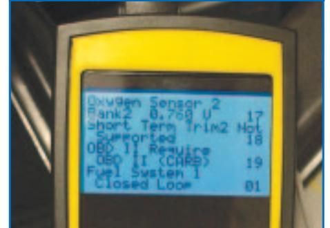
Everything seems fine until you notice that the A/F sensor voltage PID on your scan tool is exactly the opposite of what you're accustomed to seeing from a conventional oxygen sensor. The voltage output through the PCM's detection circuit and the interpreted PID on your scanner increases as the mixture goes lean and decreases as the mixture gets richer. Don't be fooled by your scanner.
