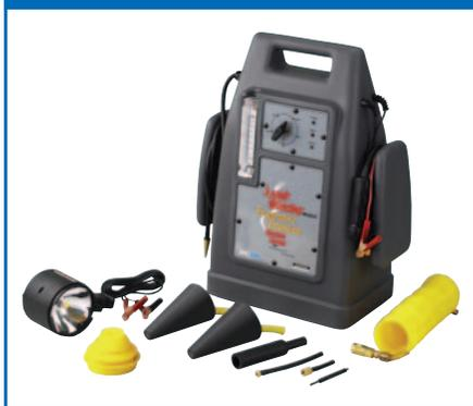
*The Vacutec EVAPro is calibrated to test systems for either .020- or .040-inch leaks. A switch position is reserved for a future calibration, in case OBD II EVAP testing gets tighter.*
